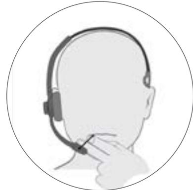
You can position the mic correctly by holding the speaker securely to your ear with one hand and adjusting the boom arm with the other until the mic tip sits two finger-widths from the corner of your mouth. Avoid positioning the mic in front of your mouth to prevent breath noise on the call.
